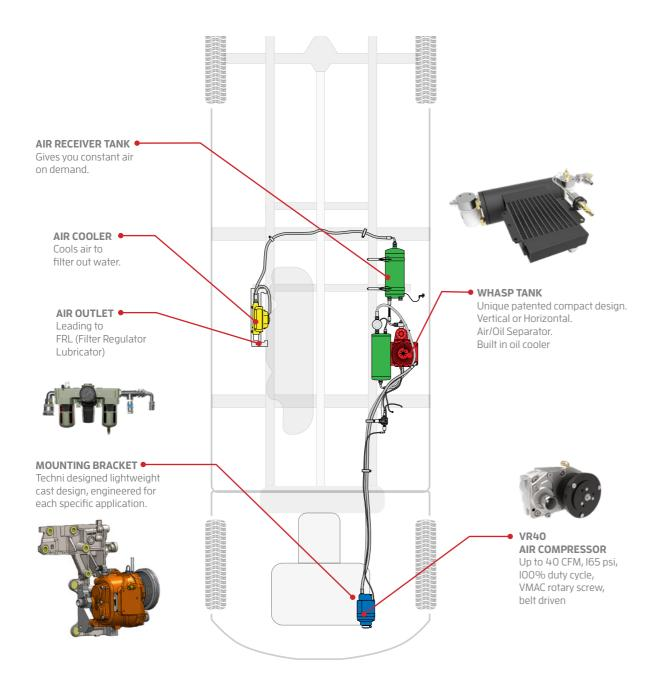
When no air is being used the system will shut off and automatically restart once tools are used and air is required. This lowers fuel consumption, emissions and noise pollution.
